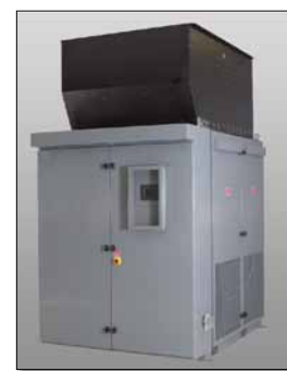
2500 kW Outdoor Stationary Resistive Load Bank – The unit is cooled vertically by a motor driven cooling fan that pulls in cool air from the lower part of the enclosure and exhausts the hot air out the top through a rain shedding exhaust hood.
